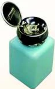
The wipe-off technique is widely used in Penetrant Inspection. The dispenser makes applying the solvent to a cotton swab or brush much easier and in a controlled manner. The integral pump delivers a small controlled amount of liquid to the cup at the top; thus reducing the evaporating rate of the remaining solvent. It keeps the bulk solvent clean, thus ensuring a clean supply of solvent to the swab or brush every time the solvent is punched just refill the dispenser.
