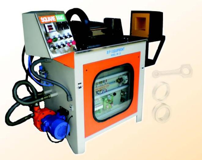
SQUAREMAG wet horizontal magnetic particle inspection equipment is used as a Multi-mode testing for surface and subsurface inspection on critical industrial and aerospace components. AC and Half Wave DC are available to meet test specifications.
