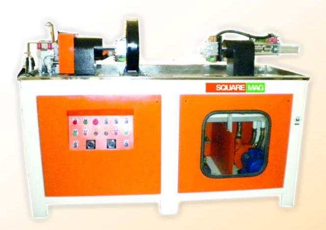
SQUAREMAG Wet Horizontal MPI Bench units provide outstanding defect detection and provide major time and cost savings over conventional magnetic testing methods. By providing combination magnetization of the part in multiple directions. virtually all defects can be revealed without having to process the part with a separate head shot and coil shot, which is the case with conventional
