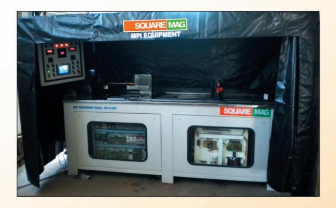
SQUAREMAG Wet Horizontal MPI Bench units provide outstanding defect detection and provide major time and cost savings over conventional magnetic testing methods. By providing combination magnetization of the part in multiple directions, virtually all defects can be revealed without having to process the part with a separate head shot and coil shot, which is the case with conventional
